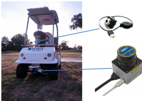
Fig.1 System layout showing Vision sensor and LIDAR.
