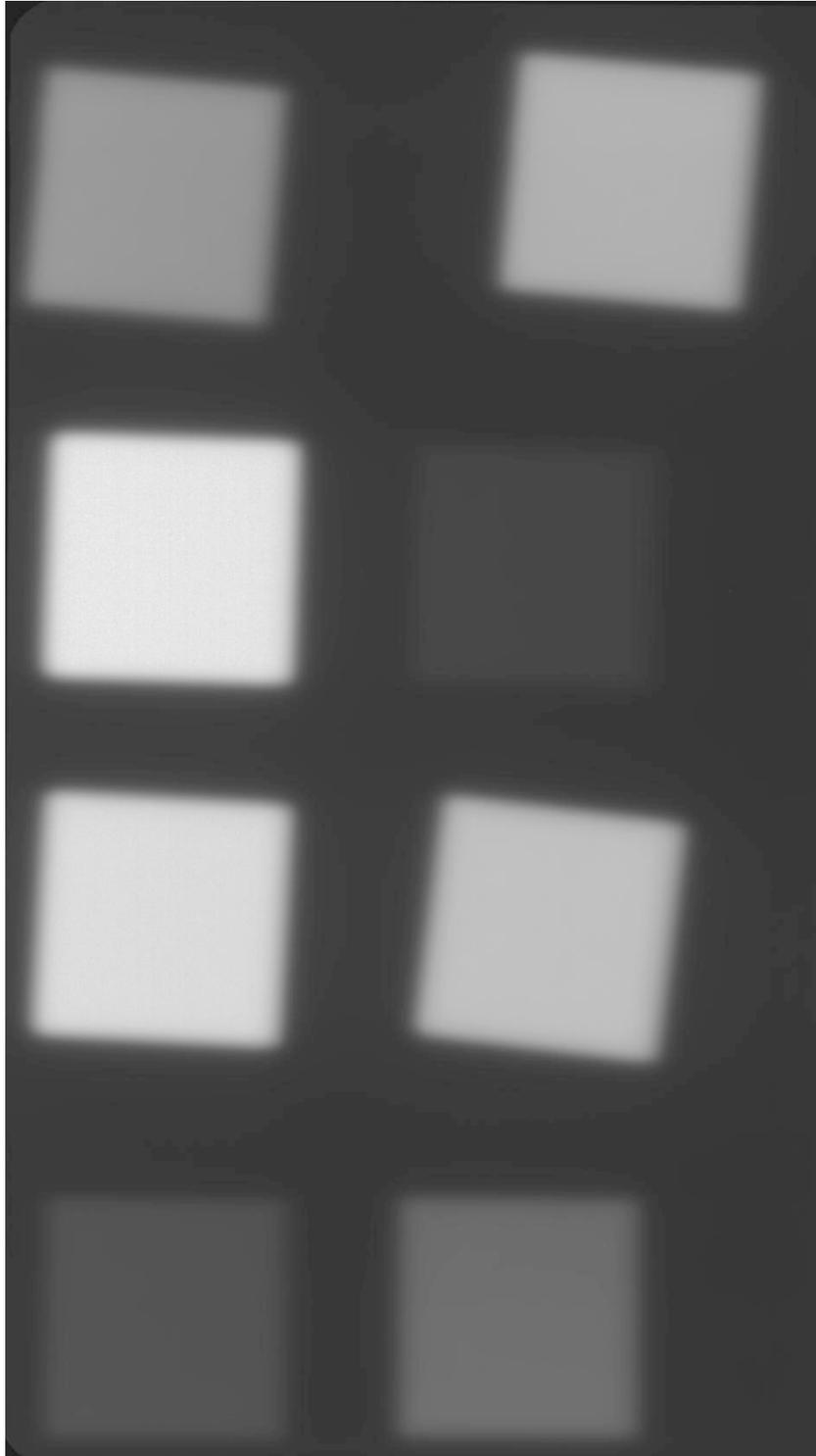
*Diagram 4.2 – the calibration film used to convert optical density to dose.*
