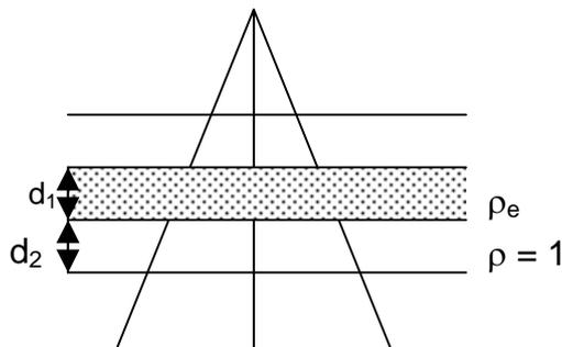
Diagram 2.3 – Setup for Batho density correction.
