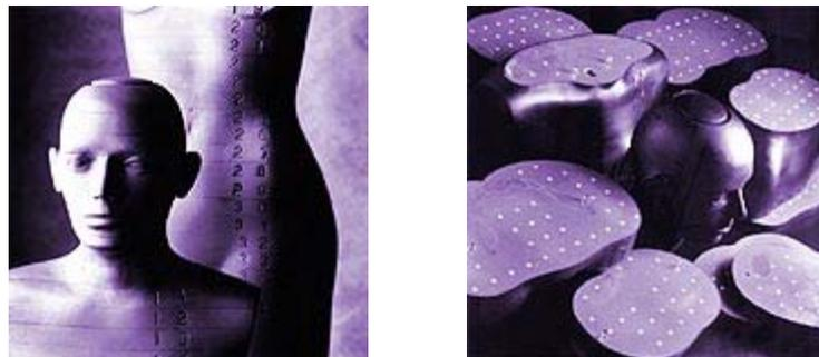
*Diagram 3.1 – Shows the RANDO™ phantom, both complete and in sections, including the slots for TLD placement.*
