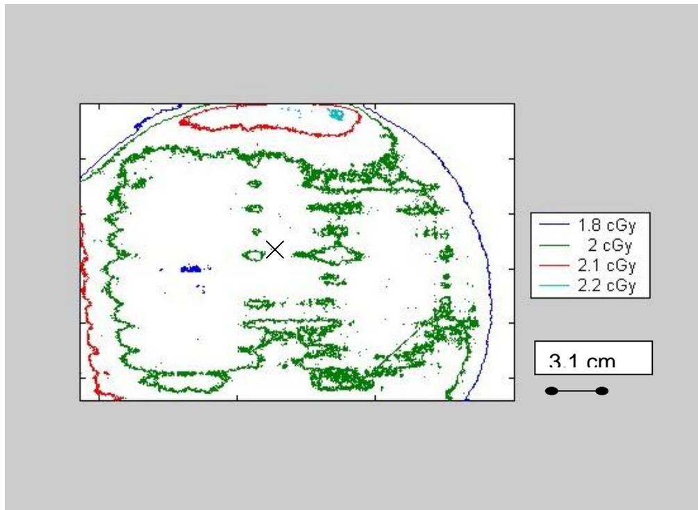
Diagram 4.7 – measured isodose distribution from film at extended SAD of 400 cm in RANDO™.
