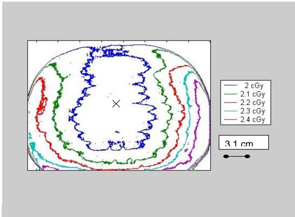
Diagram 4.6 – measured isodose distribution from film at and SAD of 100 cm in RANDO™.
