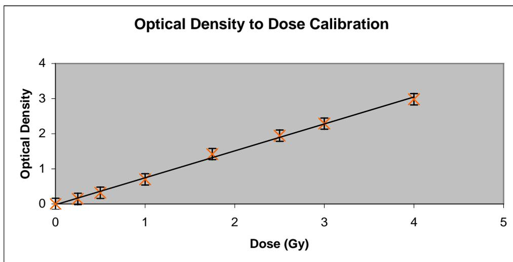
Diagram 4.3 – the calibration curve used to convert optical density to dose.
