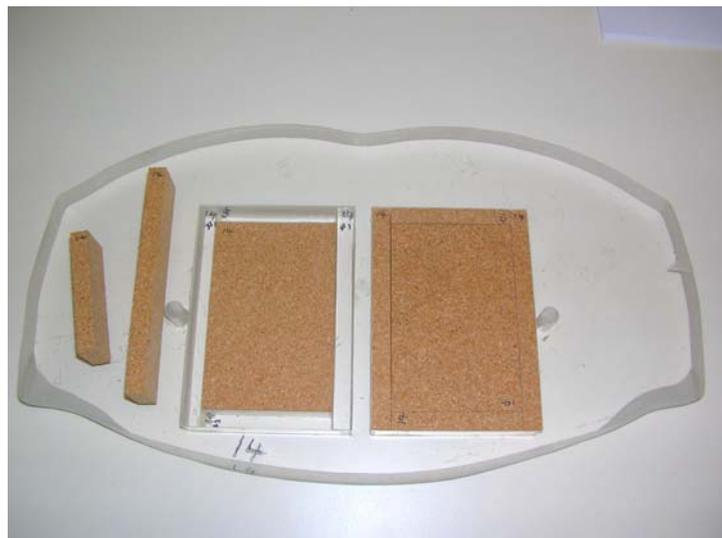
*Diagram 3.2 – a slice of the lung insert part of the anthropomorphic phantom modification showing the arrangement of the smallest lung on the left, with a cork insert surrounded by Perspex™ inserts and the largest lung, with the cork insert from the smaller lung arrangement surrounded with cork inserts, as also seen loose on the side.*
