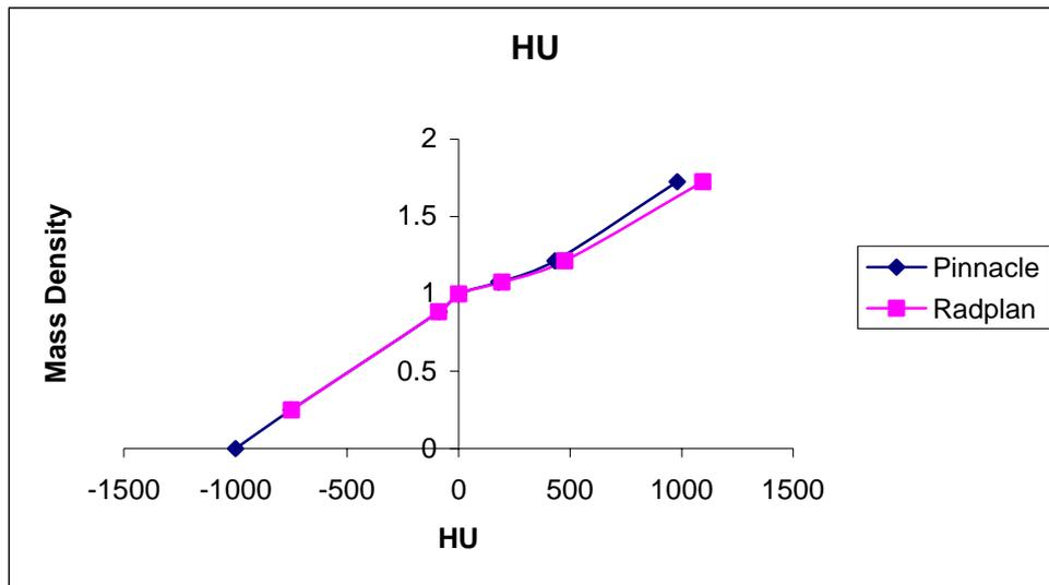
*Diagram 4.1 – the Hounsfield calibration for density used by the planning systems. The Pinnacle™ system uses CT numbers so these have been converted to Hounsfield number for display.*
