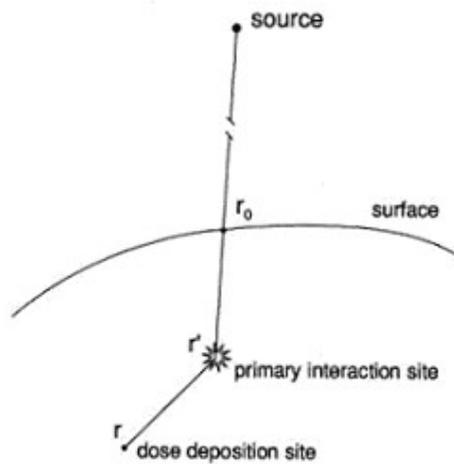
Diagram 2.5 – Shows the geometry for convolution calculation methods. (sourced from Metcalfe, Kron and Hoban, 1997)
