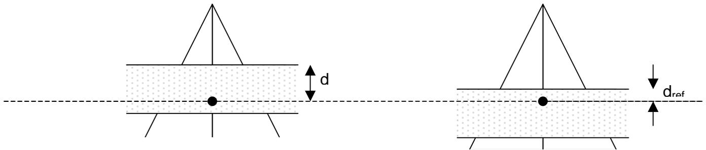
*Diagram 2.2 – Setup arrangement for measurement of TPR and TMR, where  $d$  is any given depth and  $d_{ref}$  is a fixed reference depth for TPR measurements and  $d_{max}$  for TMR measurements.*
